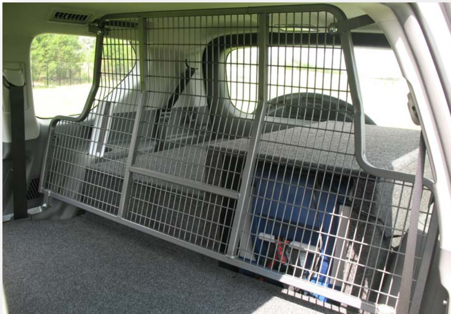
GU Nissan Patrol with Dual Position Full Cargo Barrier “Dual position” means the barrier can be fitted behind the drivers seat if required. The forward position assumes seats are folded up.
