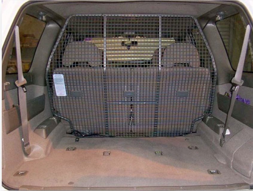
GU Nissan Patrol with Dual Position Full Cargo Barrier “Dual position” means the barrier can be fitted behind the drivers seat if required. The forward position assumes seats are folded up.
