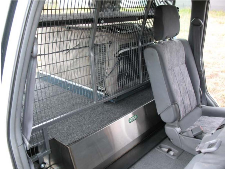
**Typical Water Tank setup behind a “Standard 2” Drawer System (100 series landcruiser)**
