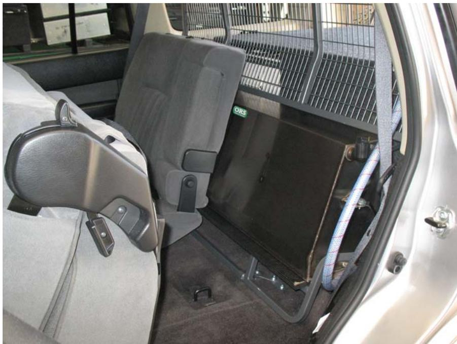
**Typical Water Tank setup behind a “Fridgepack” Drawer System (GU Patrol). Note that filling and draining the tank is all done through the rear passanger side door.**
