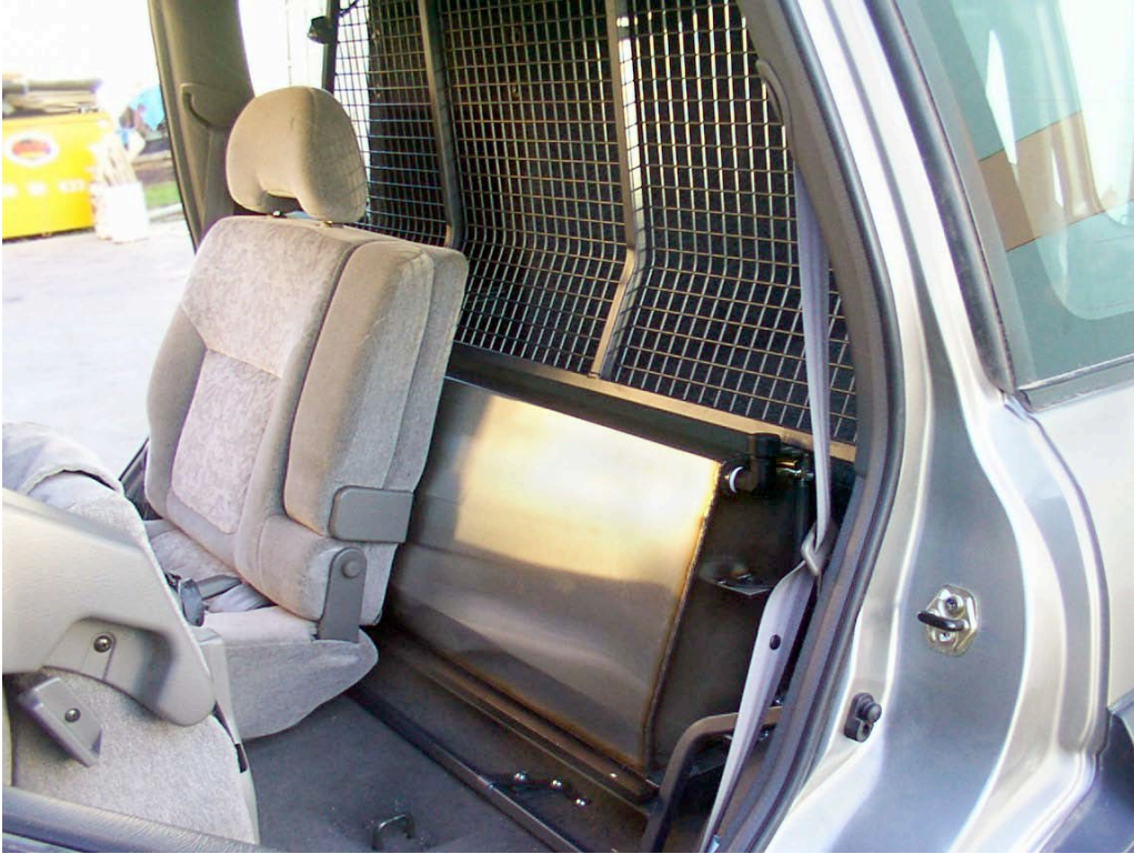
Ausguard Special Barrier with ORS 60L Water Tank This particular unit is fitted in a Nissan GU Patrol
