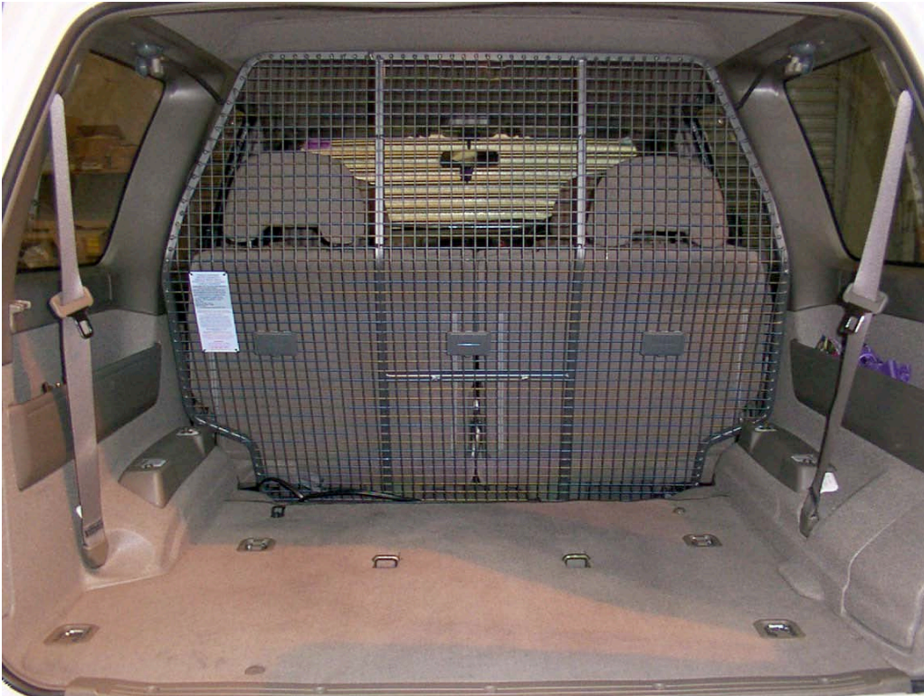
GU Nissan Patrol with Dual Position Full Cargo Barrier “Dual position” means the barrier can be fitted behind the drivers seat if required. The forward position assumes seats are folded up.
